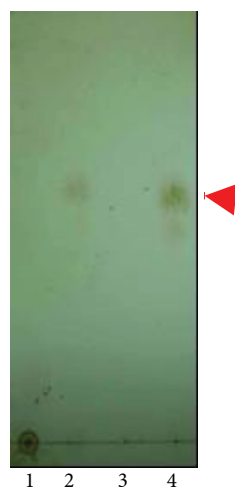
Figure 8. TLC analyses of hydrolysis products. Lane 1: purified chitinase, lane 2: hydrolysis products of colloidal chitin after 96 h, lane 3: 0.5% (w/v) of colloidal chitin, lane 4: N-acetyl glucosamine standard.
