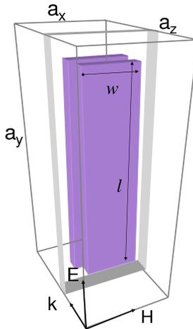
Fig. 1. (Color online) Computational configuration of a CWP unit cell.
