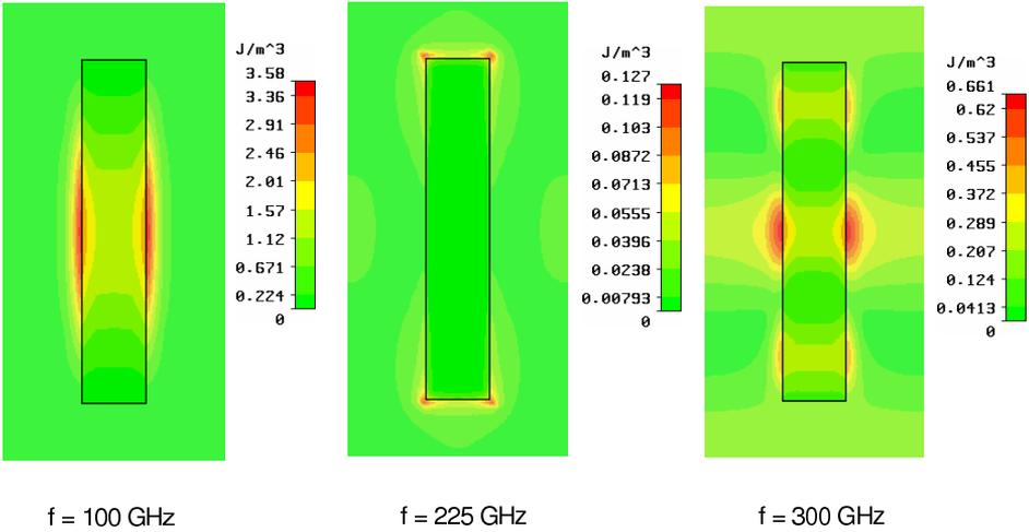
Fig. 3. (Color online) Magnetic energy distribution according to the first ( $f = 100$  GHz) and the third ( $f = 300$  GHz) resonances and the electric energy distribution for the case of second resonance ( $f = 225$  GHz).
