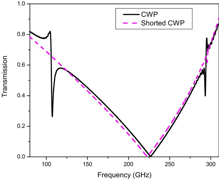
Fig. 2. (Color online) Transmission spectra of CWP and its shorted version.
