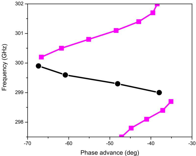
Fig. 4. (Color online) Dispersion curve for CWP structure at the polarization indicated in Fig. 1. The second branch (black curve with circles) corresponds to the negative phase velocity range.
